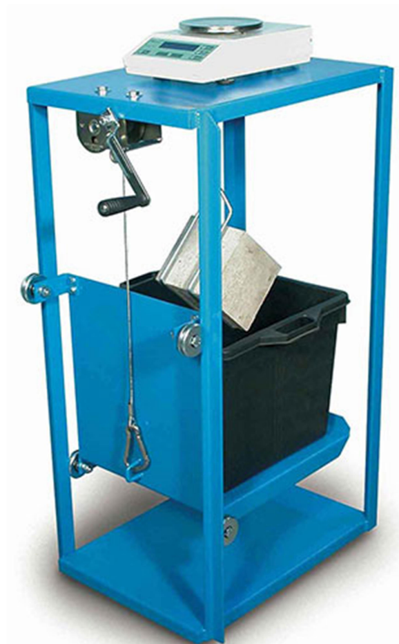
Density Of Fresh And Hardened Concrete
