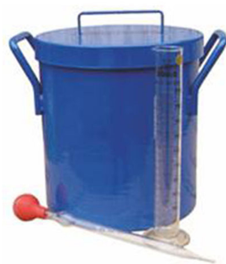
Bleeding Of Freshly Mixed Concrete
