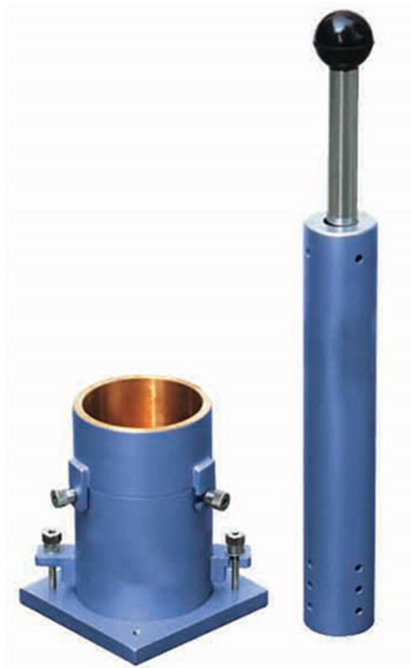
Heavy Compaction Test
