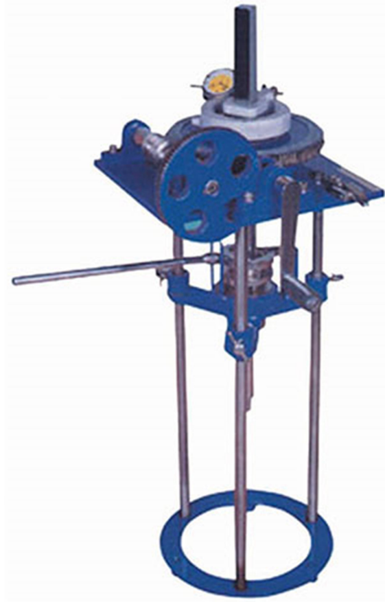
In-Situ Vane Shear Test
